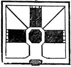
In the Gaol and Bridewell for the City of Exeter, the wings are attached to the central building, which contains the keeper's apartments, and from which there is inspection over the prisoners' airing-courts.
