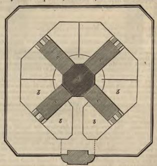
In this prison the four radiating buildings are attached to the central house (a), which contains the keeper's apartments and the chapel; from this station the eight intermediate courts (b, b, b, b) are under good inspection. The four wing-buildings had passages running through them lengthways,
